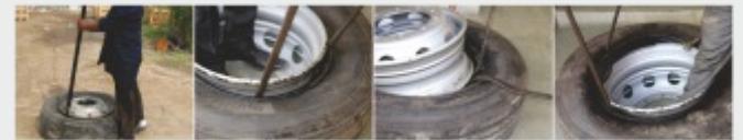
58 Tubeless Tyre Mount/Demount Regular Tool Kit
